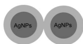
Fig. 1 Insulator shell (light grey) on conductive Ag nanoparticles (dark grey) defining the minimum distance between the cores as twice the shell thickness.
